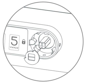
9 Insert the knob at locked position and rotate to verify that the cam stop was positioned correctly. Confirm that your mechanism is locked when the knob matches this status.
