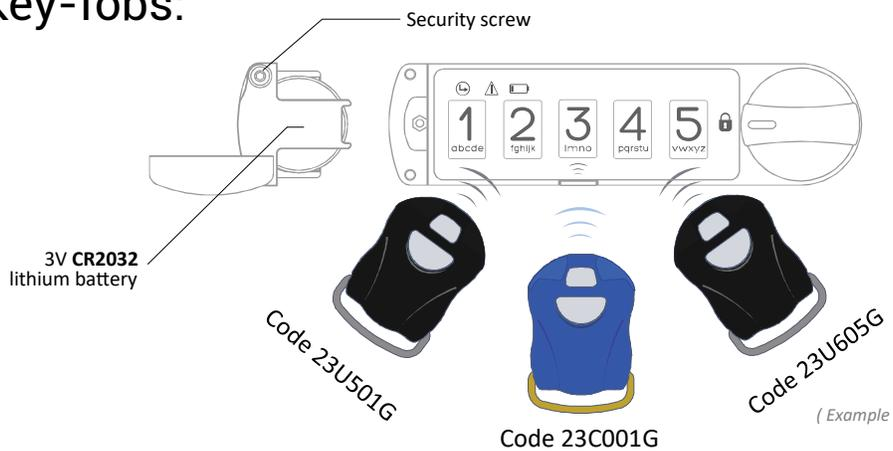
The **MicroIQ** can pair one control key fob and two user key fobs simultaneously.
