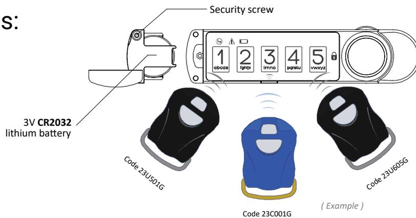
The MicroIQ lock can pair one control key fob and two user key fobs simultaneously. Multiple key fobs of the same code can be used to access the lock.
